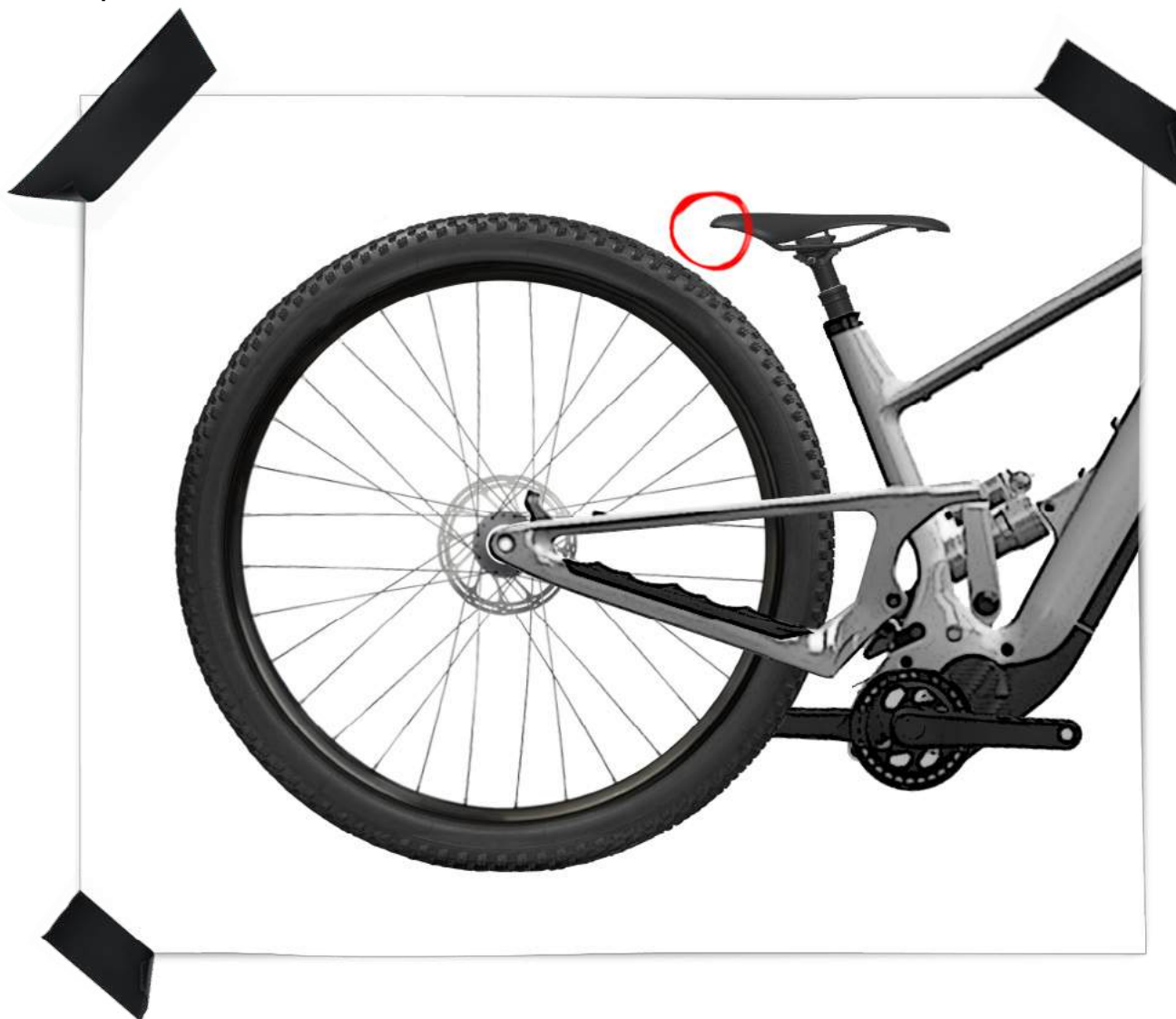
Fig.4 – saddle clearance at full compression
